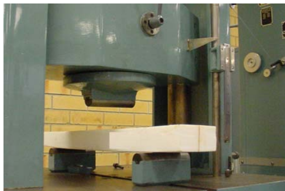
(b) Laminated wood reinforced PU foam
