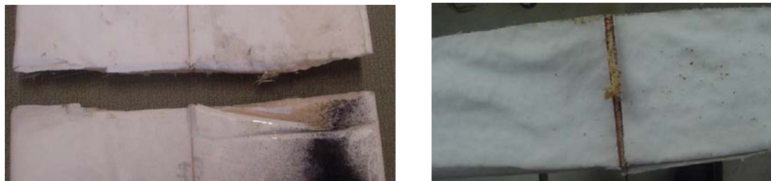
Figure 3 Photographs showing compression wrinkles across the laminate on the bottom side of a surfboard, left, and clear snapped failure due to flexural bending impact.
